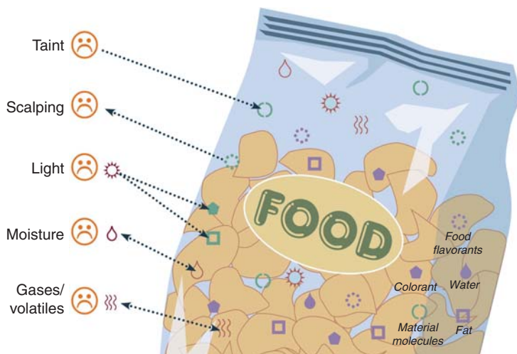
FIGURE 2.2 Negative sensory impacts occur when tainting or scalping occur or ineffective packaging selections are made.
